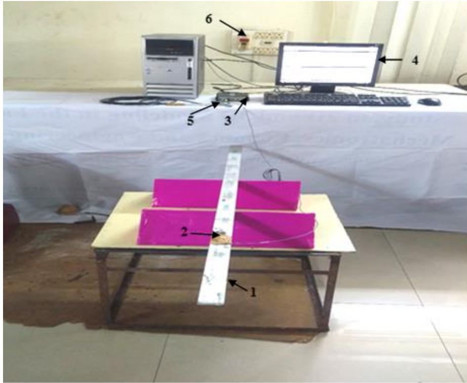
Figure 3. Experimental set up. (1-Cracked beam, 2-Vibration pick-up, 3-Vibration analyzer, 4-Vibration indicator, 5-Impact Hammer, 6-Power source)
