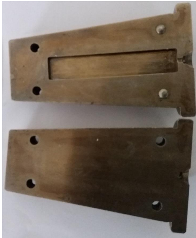
Figure 1. Mould for the ABS/MWCNT specimen.
